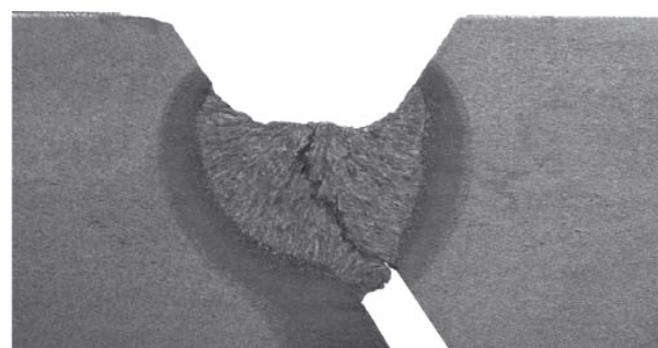
Fig. 3. Cross-section of the W1 (S500M) test joint with the visible crack initiated in weld root
