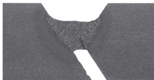
Fig. 5. Cross-section of the P12 (S500M) test joint with the visible crack initiated in weld root
