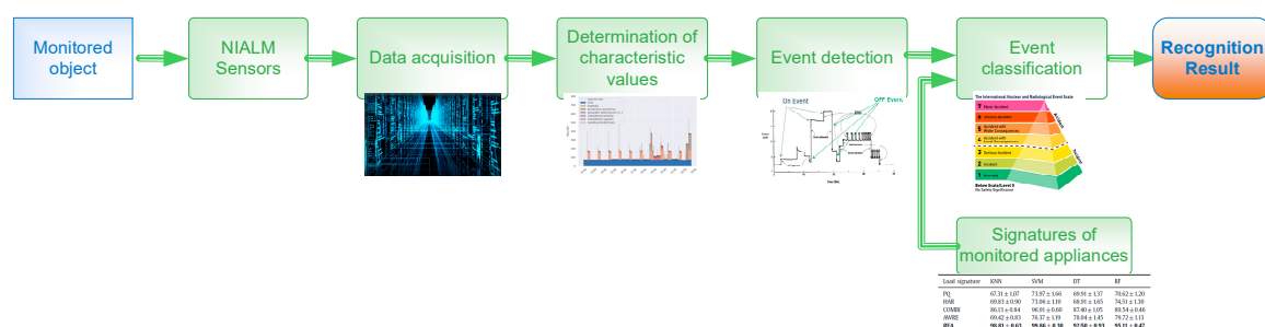
Figure 2. An example architecture of the NILM system.
