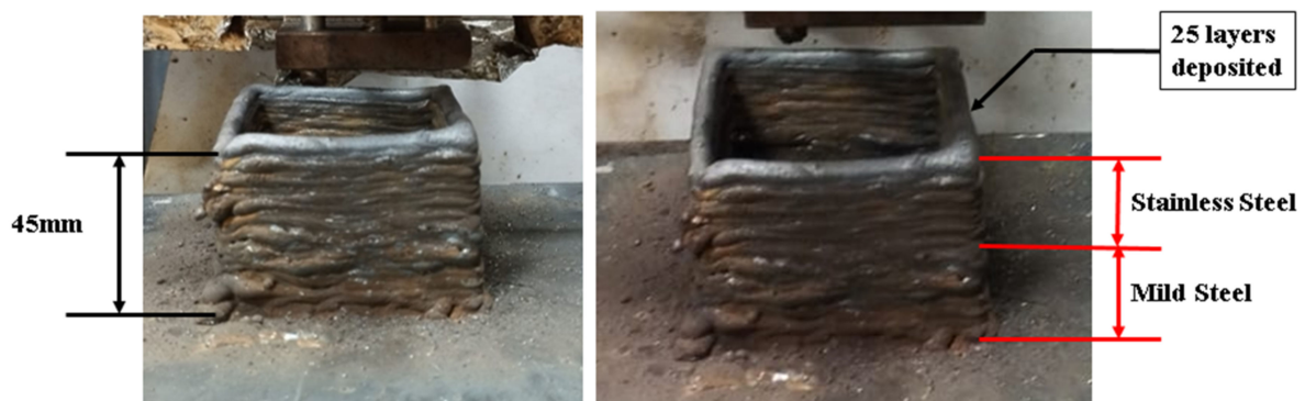
Figure 12. Mild steel and stainless steel bimetallic deposition.
