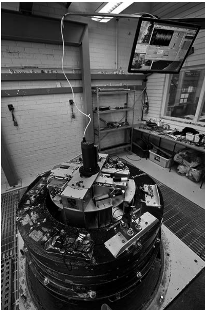
Rys. 3. Wirówka bębnowa, Centre for Offshore Foundation Systems (COFS), University of Western Australia, Perth [6; za zgodą COFS]
