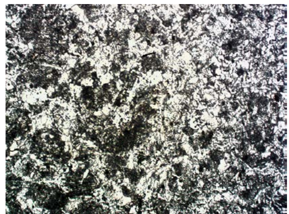
Fig. 9. Microstructure of the HAZ in joint M01; etchant: Nital; mag. 200x
