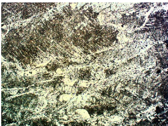
Fig. 7. Microstructure of the weld in joint M01; etchant: Nital; mag. 200x
