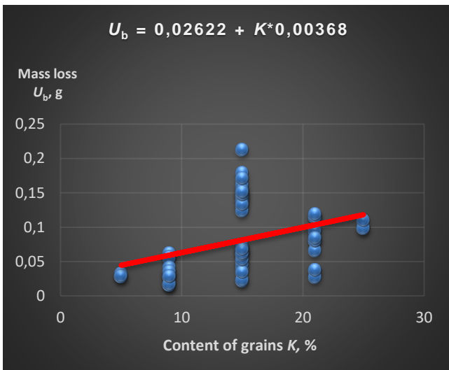
Fig. 6. Influence of abrasive grains content in the abrasive substance on the U_b cavity of Al_2O_3 ceramics during lapping (during 20 min)
