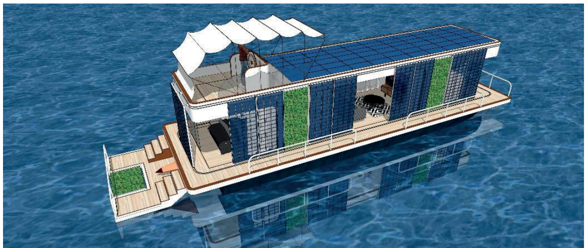
Fig. 4. Image of the proposed houseboat: view of PV roof and wall panels, green walls and an ecological floating treatment wetland
