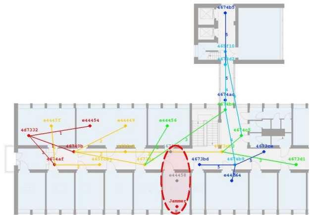
Fig. 4. Jammer placed in a closed space (room), jamming signal power level set to -11 dBm, 2 nodes affected
