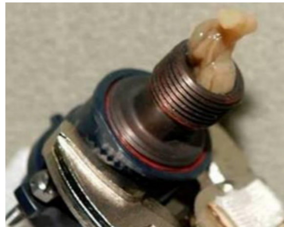
Fig. 3 - An example of biofilm formation located at the inlet to Russian condensate processor. Photo: NASA [9]
