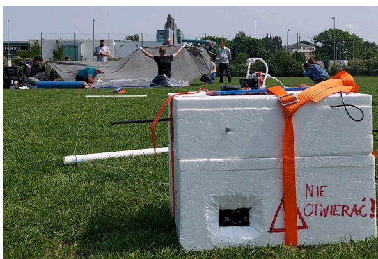
Fig. 4: Gondola made out of Eurobox-style Styrofoam boxes; rigging and launchpad visible in the background.
