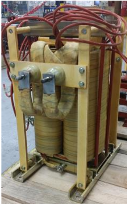
Fig. A1. Single-phase MFT prototype 180 kVA [139]
