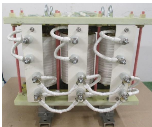
Fig. A8. 3-phase MFT prototype T2 before impregnation
