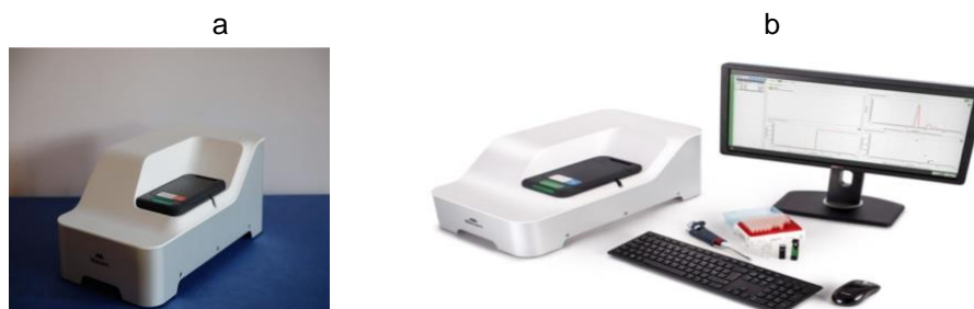
Figure 2.32 zetasizer device for measuring particle size distribution and zeta potential. (Figure source, Malvern instrument)
