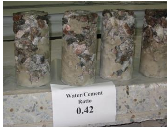
Figure 2. Shown the grout has failed to propagate through aggregate skeleton.
