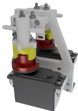
Fig. 7. Valve Control Unit
