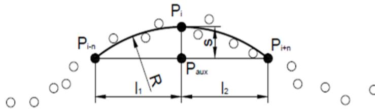
Figure 4. A diagram of track curvature calculation using satellite measurements.
