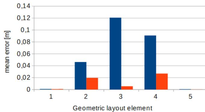
**Figure 12.** Absolute values of the mean matching error: blue bars—before the correction, red bars—following the correction, 1—straight line 1; 2—super-elevation ramp 1; 3—circular curve; 4—super-elevation ramp 2; 5—straight line 2.
