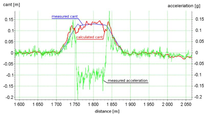
**Figure 7.** A graph of the automatically restored cant. The measured acceleration is marked in green, the calculated cant in red, and the measured cant in blue.
