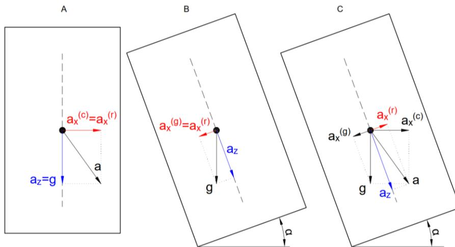
**Figure 3.** The distribution of acceleration in different movement patterns. (a) a case of movement along a circular curve without a cant, (b) a case of movement along a tangent section with a cant, (c) a case of movement along a circular curve with a cant.
