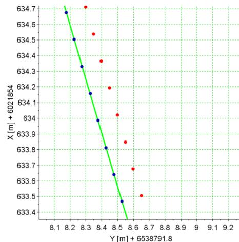
**Figure 9.** A comparison of the location of measured and corrected coordinates and the theoretical location of the track axis.
