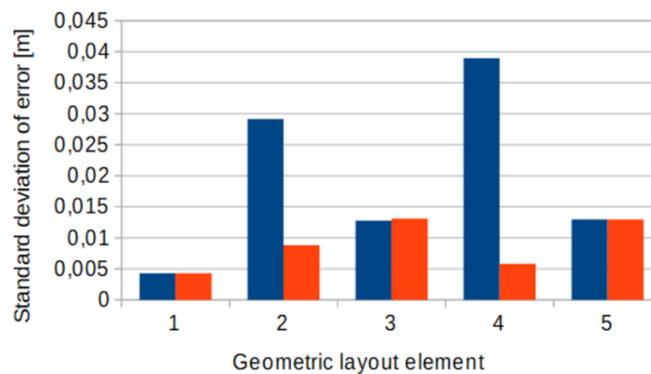
**Figure 13.** Values of the matching error standard deviations: blue bars—before the correction, red bars—following the correction); 1—straight line 1, 2—super-elevation ramp 1; 3—circular curve; 4—super-elevation ramp 2; 5—straight line 2.
