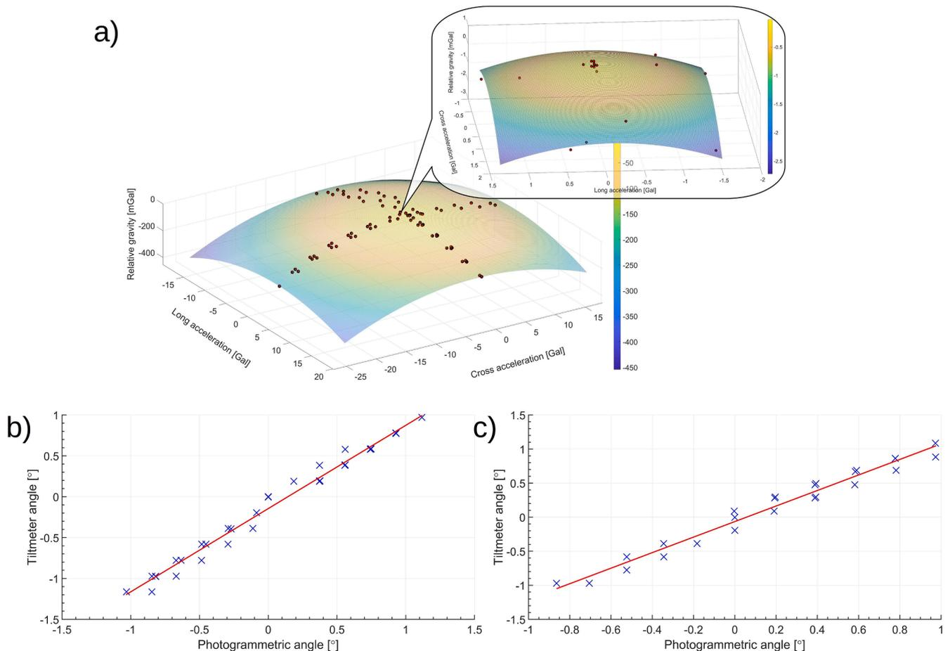
**Fig. 3.** The results of tiltmeters calibration: a) The parabolic surface fitted to the data in order to find where its maximum is located, the 2 Gal zone around maximum is magnified b) the calibration of the scale factor of long tiltmeter c) the calibration of the scale factor of cross tiltmeter.
