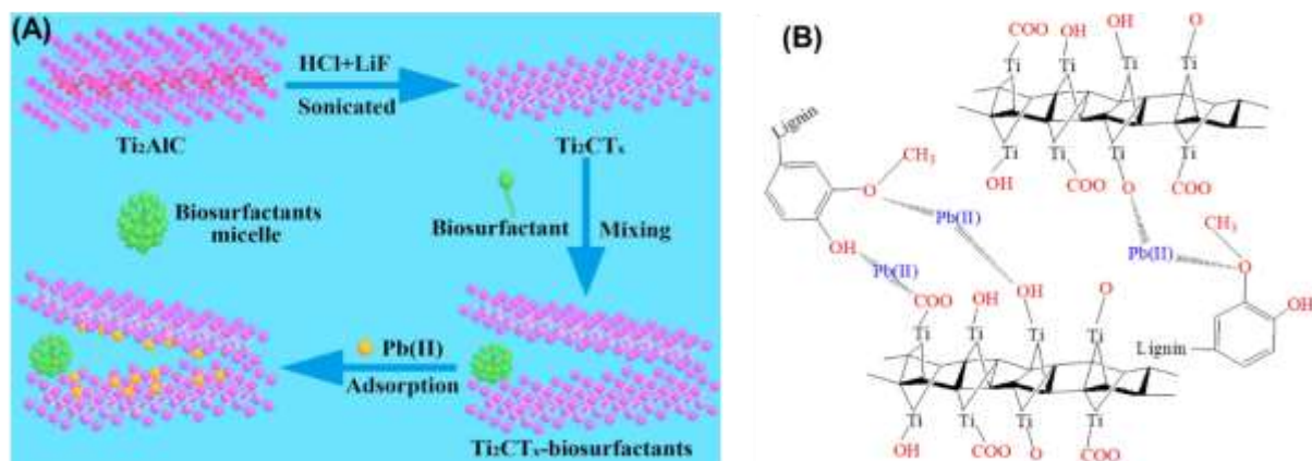
Figure 6: (A) preparation process of biosurfactant-functionalized MXene and (B) the schematic of the adsorption mechanism for Pb(II) . (Reproduced with permission from ref. [83])
