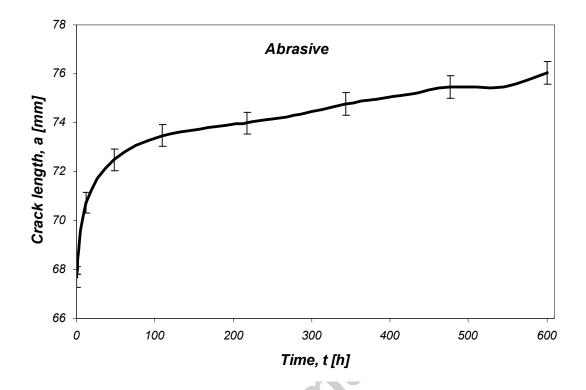
Fig. 5. Results of crack length, a, vs time, t, for wedge test with abrasive prepared surfaces.
