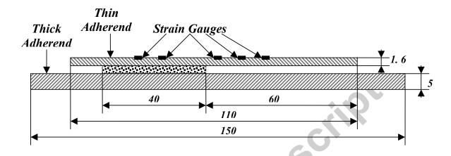
**Fig. 1.** Representation of geometry of asymmetric wedge test sample. (Dimensions in mm.)
