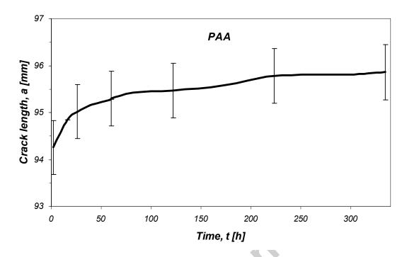
**Fig. 6.** Results of crack length, *a*, *vs* time, *t*, for wedge test with PAA prepared surfaces.
