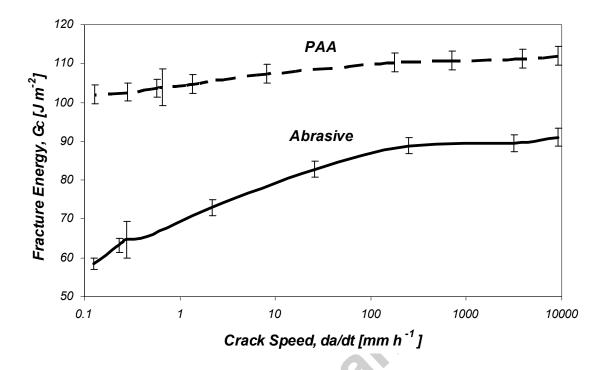
Fig. 7. Fracture, or adhesion, energy,  $G_c$ , vs crack growth rate, da(t)/dt, for wedge tests after abrasive and after PAA surface treatments prior to adhesive bonding with epoxy resin. Smaller error bars are only representative and could be calculated for any value of da(t)/dt. They correspond to the result of errors *only* on a. The two larger bars, one on each curve, represent overall errors taking into account systematic effects of E,  $\Delta$  and h.
