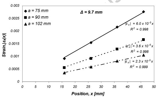
**Fig.4.** Surface strains,  $|\varepsilon_s(x)|$ , obtained from strain gauge measurements, vs positions, x, of strain gauges (x = 16, 26, 36 and 46 mm) and corresponding linear regression lines, for wedges of both thicknesses, 4.6 and 9.7 mm. The three lines in each graph correspond to imposed "crack lengths", a, given in the left upper corner.
