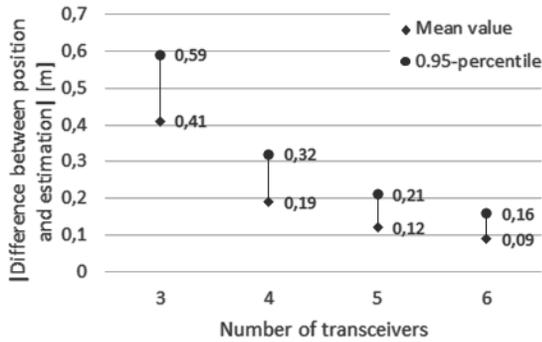
Fig. 6. Positioning accuracy vs. number of transceivers.
