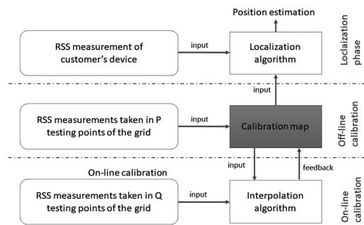
Fig. 2. Phases of the proposed fingerprints localization method.
