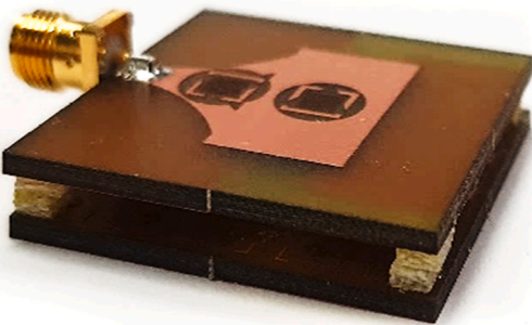
Fig. 15. Photograph of the assembled sensor prototype: perspective view.
