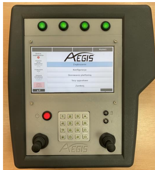
Fig. 5. The front panel of the manipulator.
