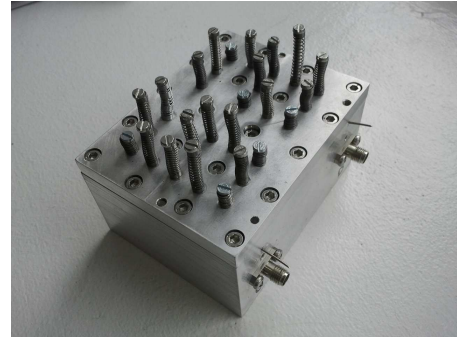
Fig. 13. Manufactured prototype of combline diplexer.
