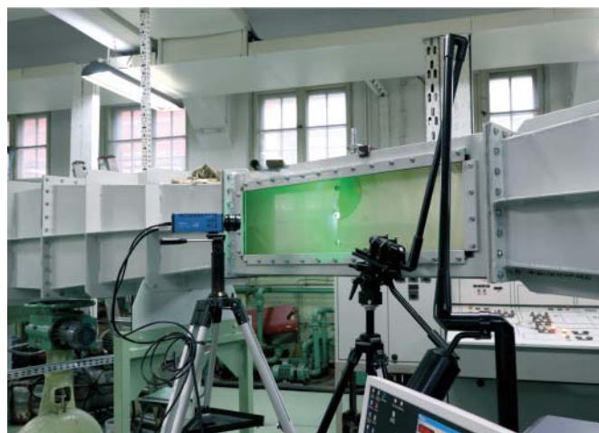
Fig. 2. Cavitation tunnel during PIV measurements
