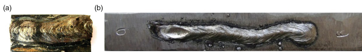
FIGURE 3. View of exemplary test weld beads: (a) mercury method (EB1.46 electrode, air welding) and (b) glycerin method (ER2.46 electrode, underwater wet welding).
