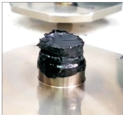
Fig. 2. The condition of bitumen samples after LAS test: a) cohesive failure inside the sample, b) flow inside the sample, c) intermediate state between cohesive damage and flow inside the sample, d) no distress – view after removal of the upper rheometer plate
