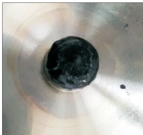
Fig. 2. The condition of bitumen samples after LAS test: a) cohesive failure inside the sample, b) flow inside the sample, c) intermediate state between cohesive damage and flow inside the sample, d) no distress – view after removal of the upper rheometer plate
