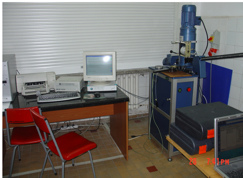
Fig.1 Schematic diagram of the ITeE Radom company four-ball tester and the Vallen-Systeme GmbH AMSY-5 apparatus measurement and control systems[1]
