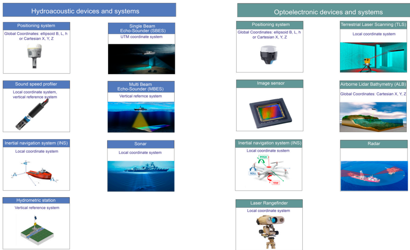
Figure 1. A diagram presenting hydroacoustic (blue colour) and optoelectronic (green colour) devices and systems.
