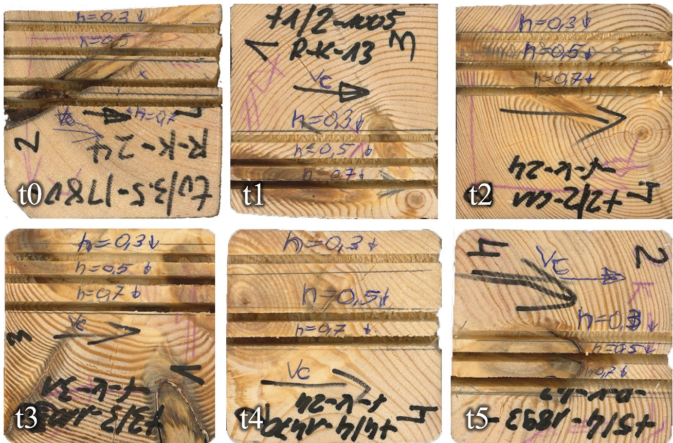
Fig. 2 Cross section of the knotty wood side. Three grooves were cut on each of the six cross sections. Cutting direction was left to right, as shown in the picture. The markings on the cross sections are only for
