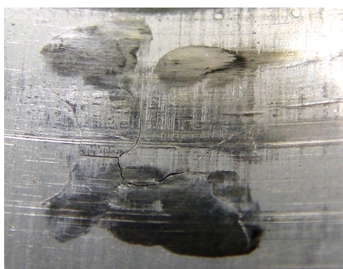
Fig. 8. Net of cracks on the sliding surface of the MB58 bush (zoom out of the part of the sliding surface shown in Fig. 7b) [9]
