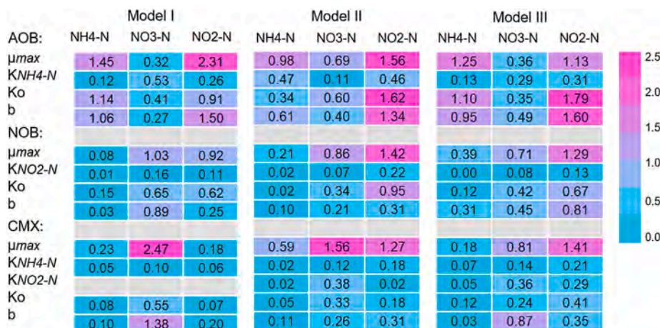
Fig. 3. Heatmap of the sensitivity coefficients for the three examined models.
