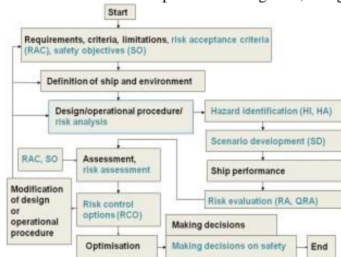
Figure 2. Structure of the method of risk and safety assessment of ships in damaged conditions.
