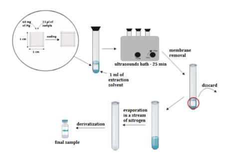
Figure 1Scheme of the ultrasound-assisted solvent extraction of porous membrane packed liquid samples extraction process.
