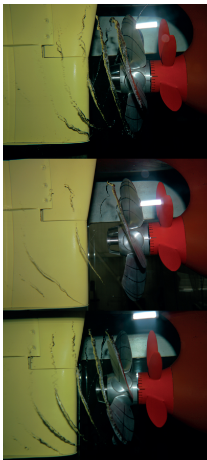
Fig. 14. Tip vortices for KT (from up to down): 0.243; 0.296; 0.361
