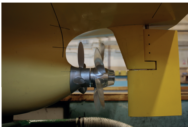
Fig. 6. Self-propulsion test arrangement with pre-swirl stator
