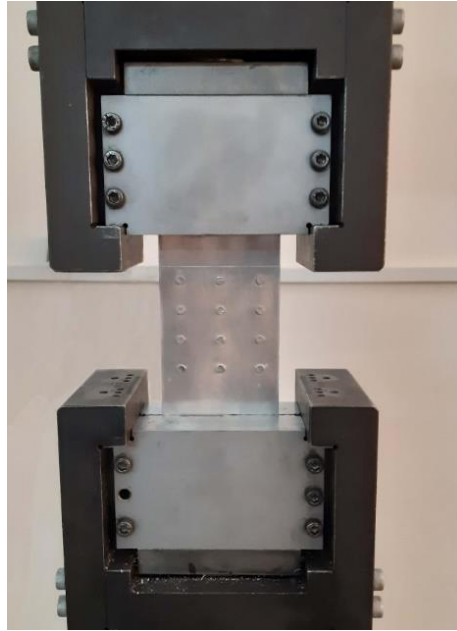
Fig. 3. Experimental test setup for fatigue life estimation.
