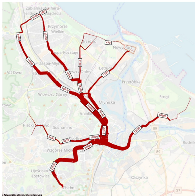
Fig. 1. Cartogram of passenger streams on Gdańsk tram network daily in 2016 (source: Gdański Model Podróży 2016 )
