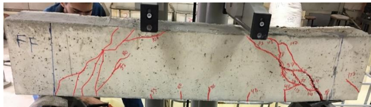
Fig.12: Beam (B4) at failure
