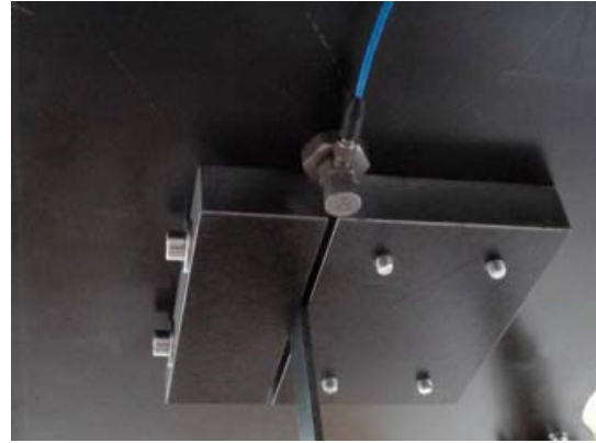
Fig. 6: Bottom part of the moving platform with top support of column and accelerometer
