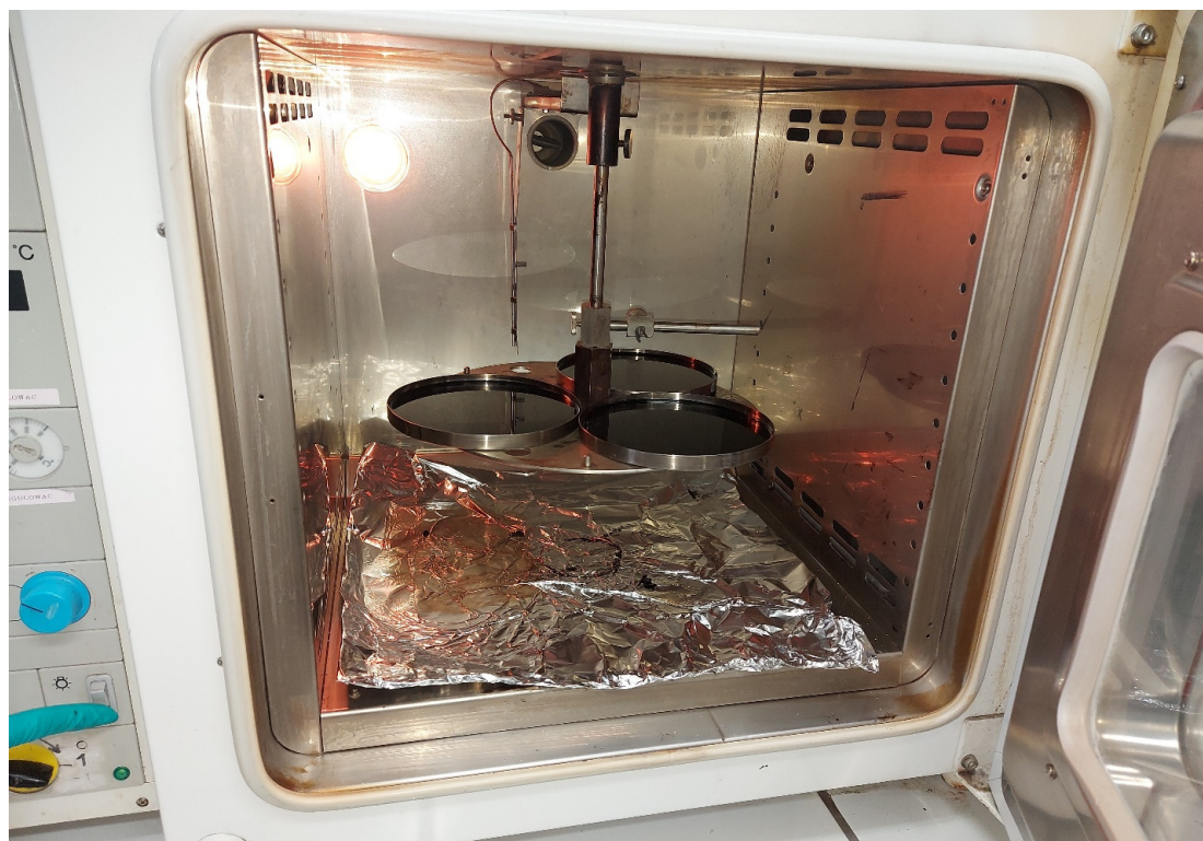
Figure 7. Photograph of a set of pans and an oven for aging bitumen by the TFOT method [own material].
