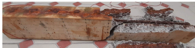
Fig. 14. Specimen after destruction with type B.
