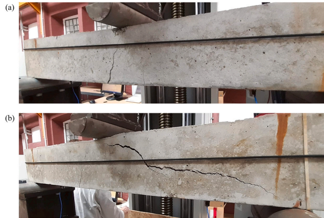
Fig. 13. Two types of failure modes: (a) type A – flexural failure, (b) type B – shear failure.
