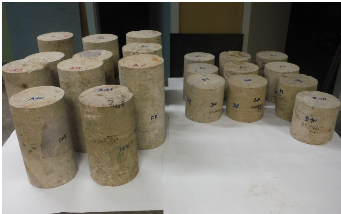
Figure 1. Core samples type A and B after cut geometry preparation
