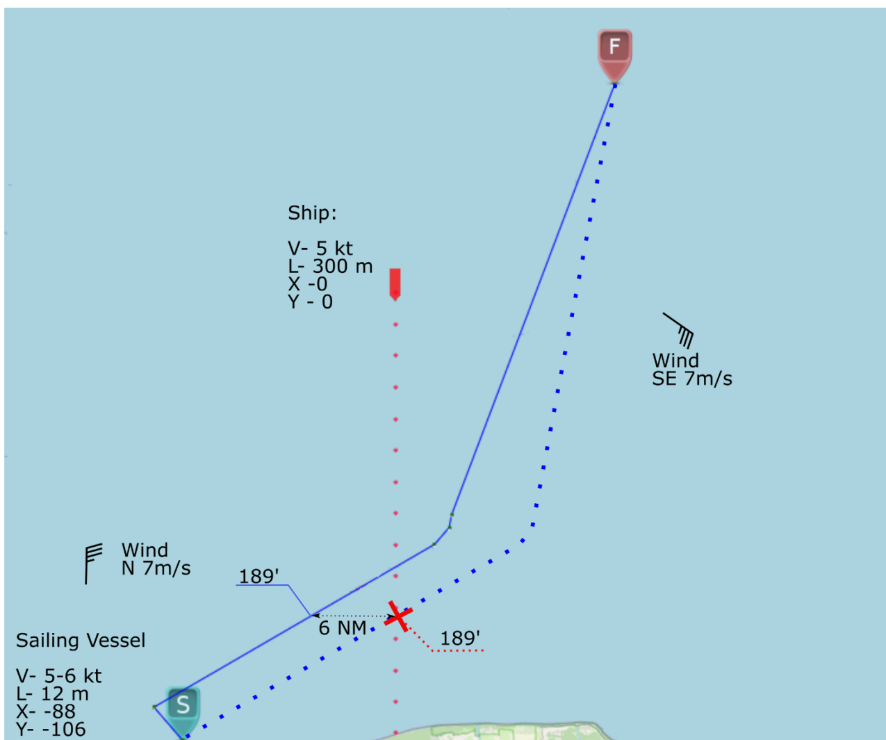
Figure 12. Scenario 1: A sailing vessel avoids collision with a power-driven ship by passing astern, which requires a substantial turn to port. Least-time route of a sailing vessel is marked as a dotted blue line, collision avoidance route – as a solid blue line and the target's path – as a dotted red line.
