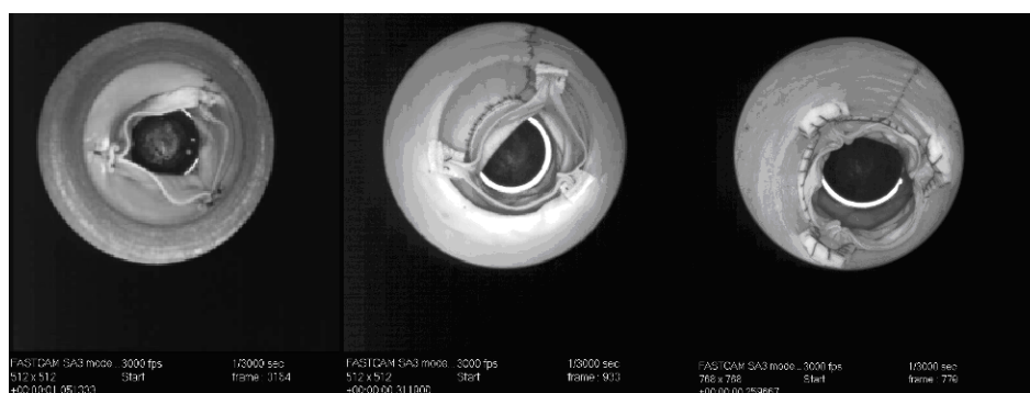
Fig. 6. Image captured by the high-speed camera showing the full opening of the implants treated with the same parameters of the flow. On the left: HAB_1, Reference_1, Reference_2.
