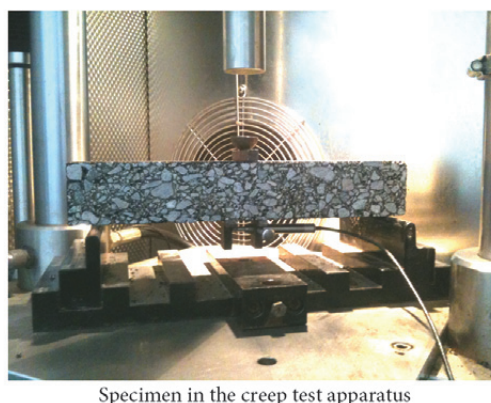
Fig. 3. Bending creep test – the test setup
