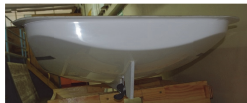
Fig. 9 Model without appendages during the test
