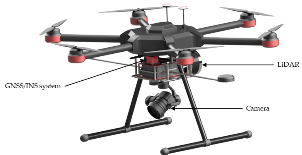
Figure 6. A concept of an optoelectronic module dedicated for an unmanned aerial vehicle (UAV), which will allow photogrammetric surveys in the coastal zone to be conducted.
