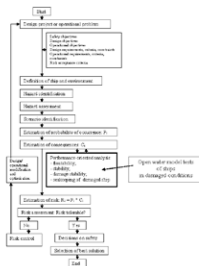
Fig. 2 Logical structure of the risk-based design/operational procedure (method).
