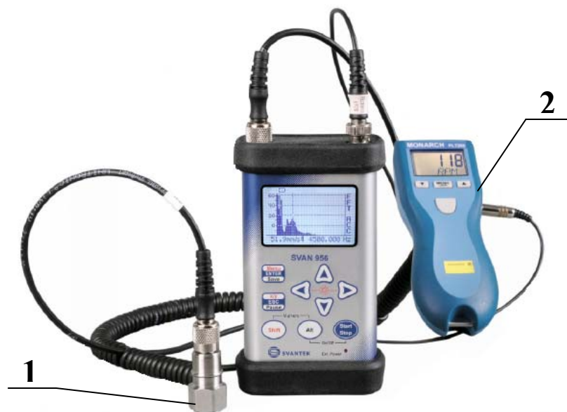
Fig. 10. Digital vibration register and analyser „SVAN 956” [24] 1 – piezoelectric sensor of vibration’s acceleration, 2 – laser tachometer probe.
