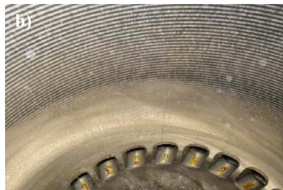
Fig. 2. Port-valve timing system of the 7L35MC-S engine a) flow diagram of the working medium, b) inlet (admission) ports.
