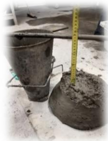
Fig.3: The slump test.
