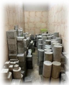
Fig.4: Curing the concrete samples.
