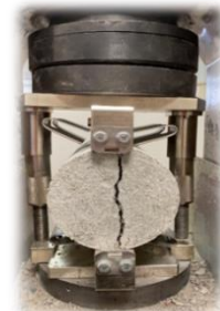
Fig.6: The splitting test.
