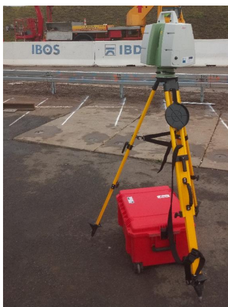
Fig. 1 Leica C10 laser scanner, placed on the tripod.
