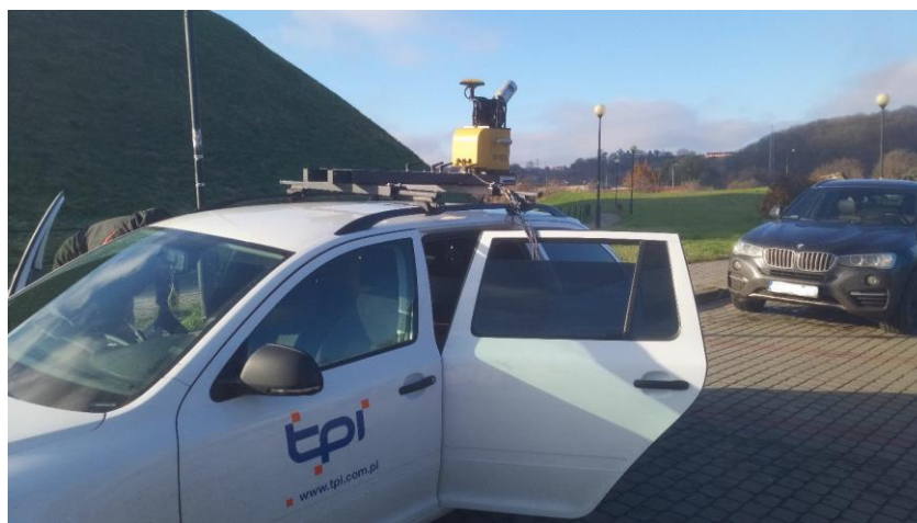
Fig. 2 Mobile laser scanner (Topcon, IP-53)
