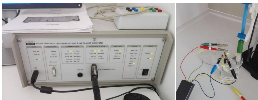
Fig. 3. Corrosion test stand
